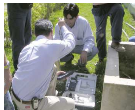
Measuring pH and EC in the field
