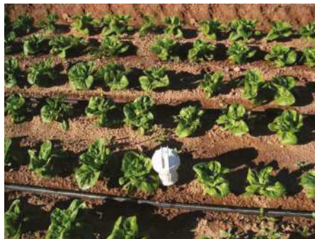
Capacitance probe in lettuce field (in operation)
