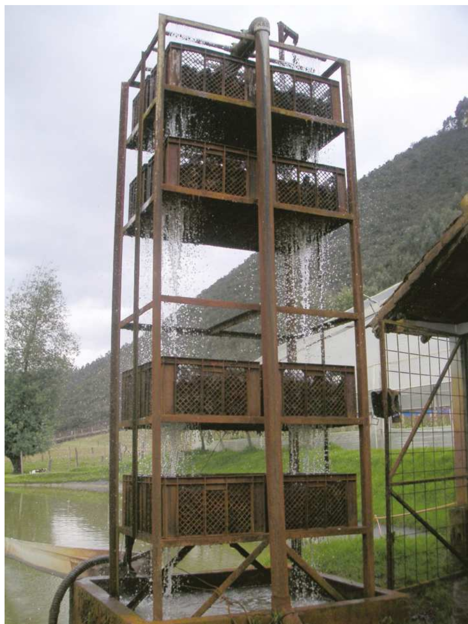
Aeration tower for irrigation water
