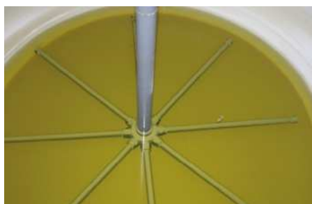
Precipitation from long term addition of micronutrients
