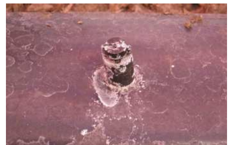
All types of drippers are liable to clogging
