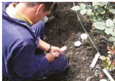
Monitoring the soil solution
