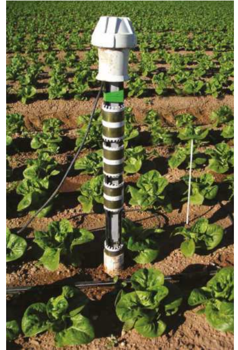
Capacitance probe in lettuce field (open)
