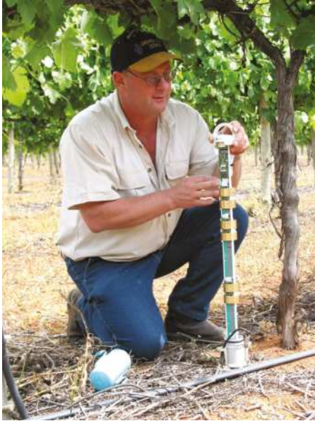
Monitoring soil moisture with a capacitance probe
