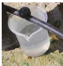
Sampling drip discharge
