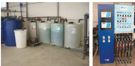
Head unit with multiple and independent tanks and injectors
