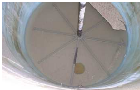
Deposit from incompatible fertilizer
