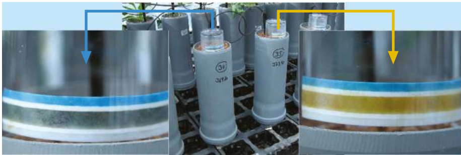
The grey color of the test strip (left) indicates high ammonia volatilization from a soil fertigated with an ammonium-based fertilizer regime. Right, low volatilization from a largely nitrate-based programme.
